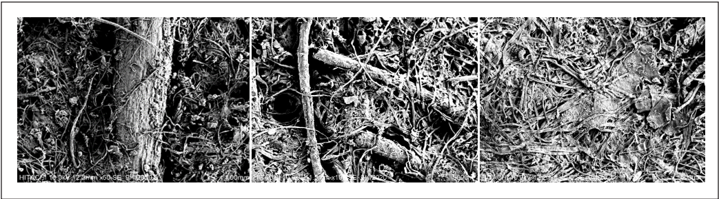
Figure 2. SEM images of OPT briquettes (left: 50×, center: 100×, right: 300×)
